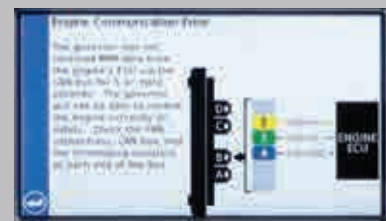
Error screen describing issue with suggested solution and illustration.
