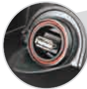
USB port for database transfer and diagnostics
